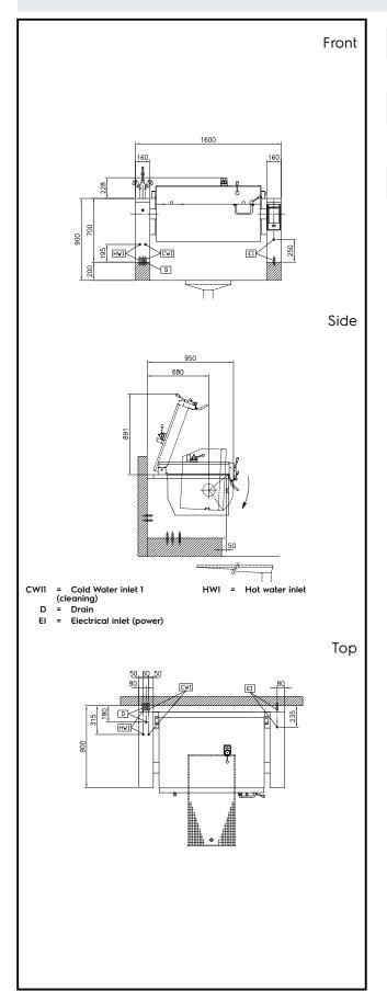
**Electric** Supply voltage: 400 V/3N ph/50/60 Hz Total Watts: 20.6 kW Installation: FS on concrete base;FS on feet;On base;Standing Type of installation: against wall **Key Information:**
